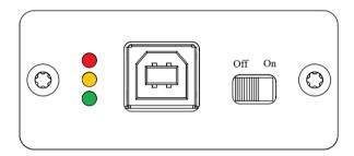
The Ecumaster USBtoCAN is equipped with a 120 Ohm terminator that can be used for CAN bus termination. If you are not using an external terminator, it is necessary to use the one provided by USBtoCAN interface, otherwise the communication will not work. The USBtoCAN terminator can be turned on or off using a switch on the casing.
